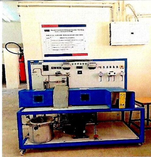
Ductable AC testing
